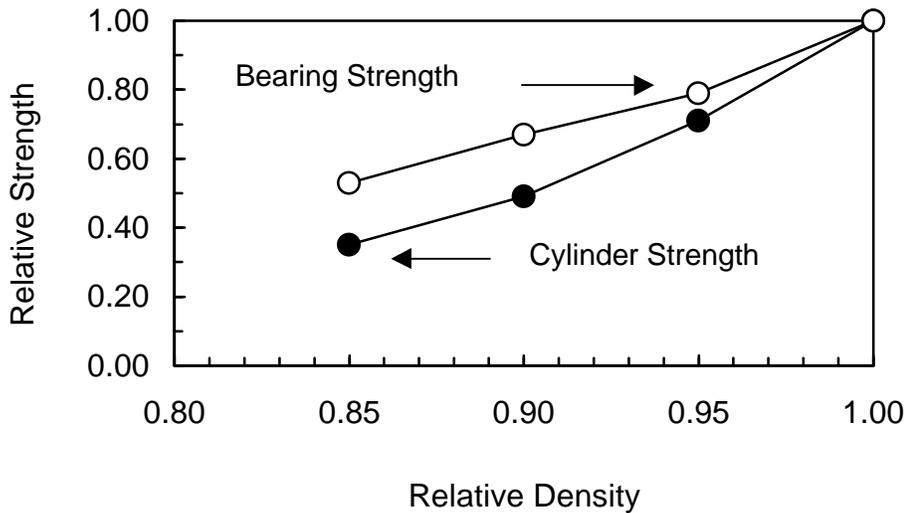
**Fig. 4: Relationship between relative strengths in compression and bearing and relative density for polystyrene aggregate concrete**
