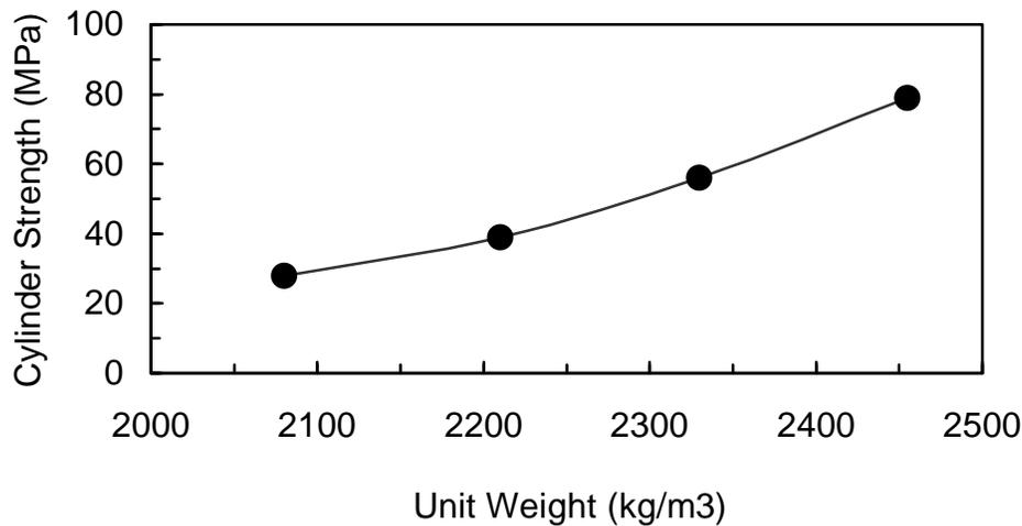
Fig. 2: Relationship between unit weight and compressive strength
