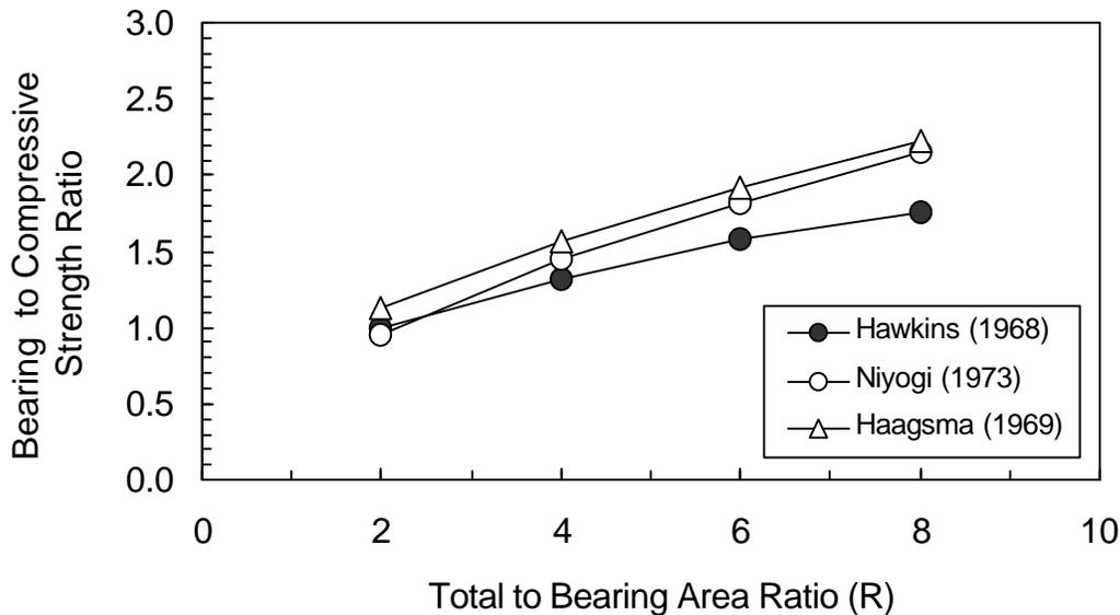
**Fig. 1: Bearing strength of normal weight concrete as a function of compressive strength and bearing area**
