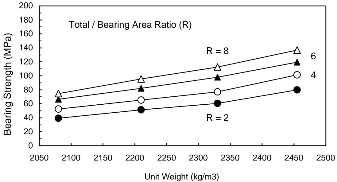
**Fig. 3: Effect of unit weight, bearing area on bearing strength of polystyrene aggregate concrete**
