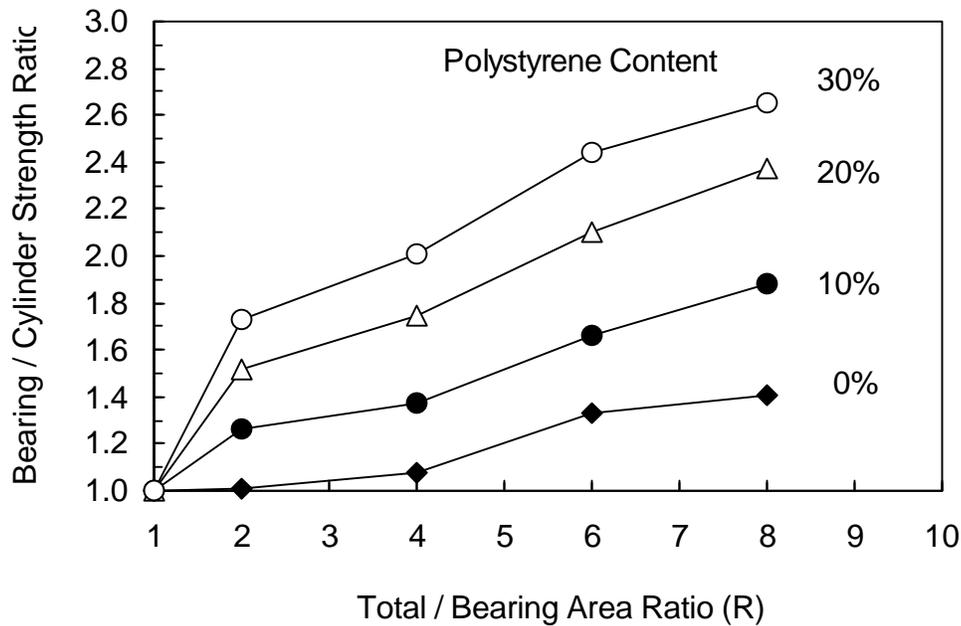
**Fig. 5: Relationship between bearing to cylinder strength ratio and total to bearing area ratio (R)**
